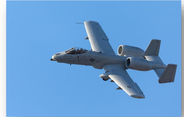
An A-10C Thunderbolt II “Warthog” flew over Florida’s Gulf Coast on June 29, 2012, marking the second flight of an aircraft powered solely by an alcohol-derived jet fuel blend (supplied by Gevo). Source: Reuters
